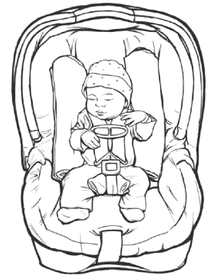
Figure 3. Car safety seat with a small cloth between crotch strap and infant, retainer clip positioned at the midpoint of the infant's chest, and blanket rolls on both sides of the infant.
